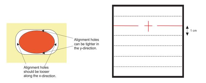
Figure 5. Alignment holes recommendation
