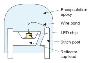
Figure 3. Common TH LED construction
