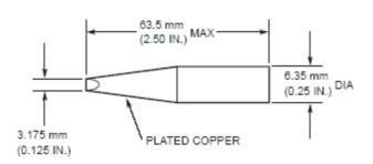
Figure 2. Example of soldering iron tip for hand soldering TH LED components
