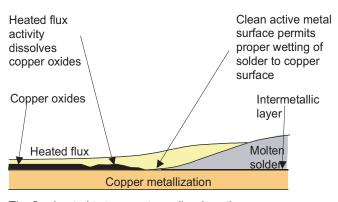
The flux heated to temperature, dissolves the copper oxides leaving a clean, chemically active copper surface and prevents further oxidation. The molten solder immediately wets the copper surface.
