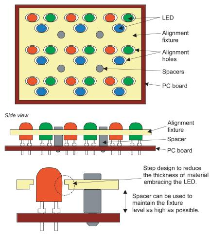
Figure 4. Illustration of the alignment fixture and spacers
