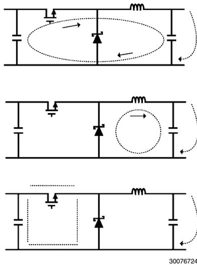
FIGURE 5. Current Flow in a Buck Application
